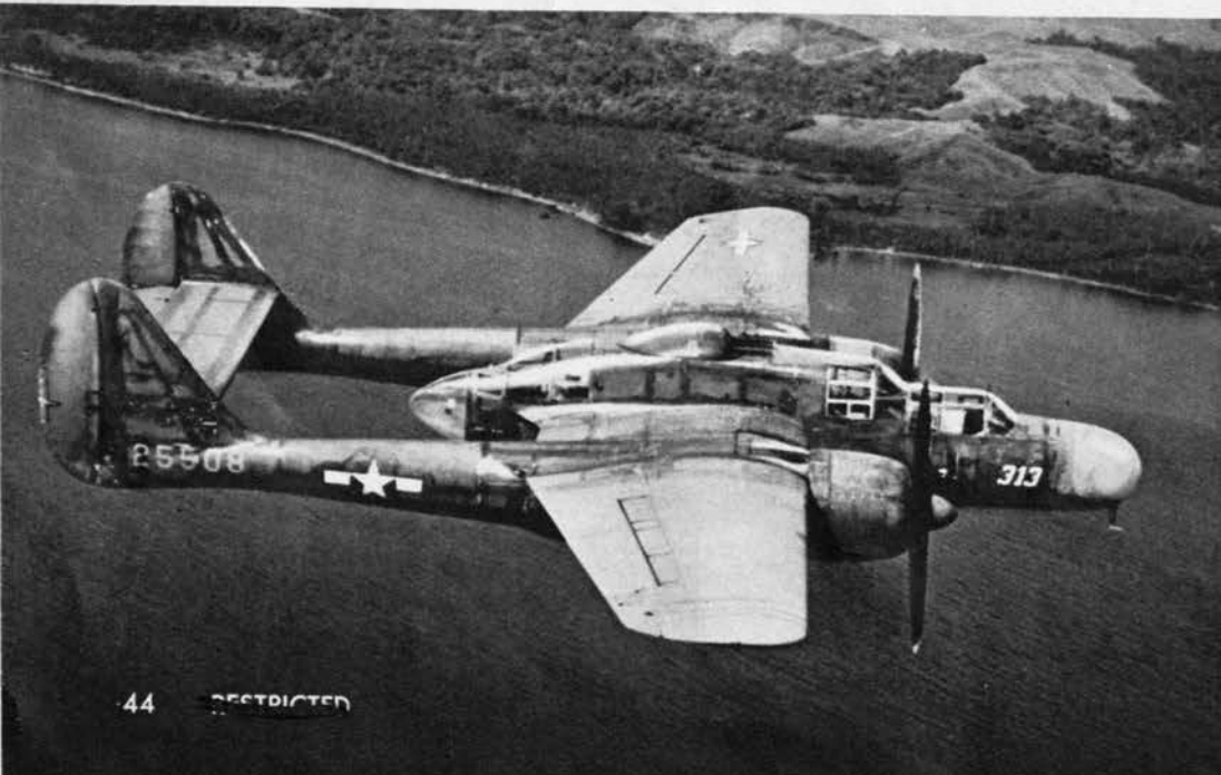
Ungainly but effective , the P-61 ( below ) is protecting our Pacific bases from Japanese night forays. Heavy gondola has three steps in front, comes to a point at the rear. The wing, which tapers only on the trailing edge, carries underslung engines and distinctive twin booms.
